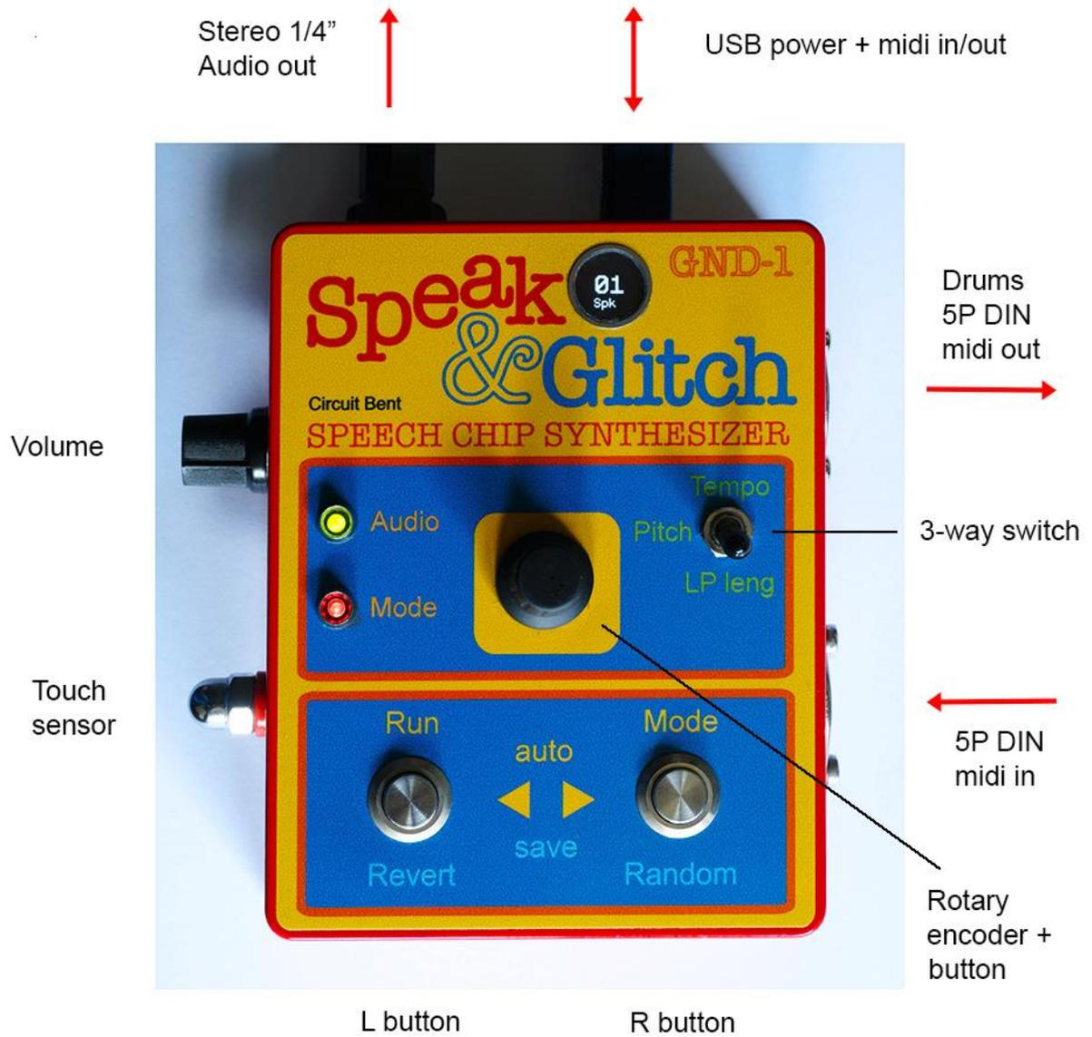
FIG. 1 GND-1 Controls and connections
